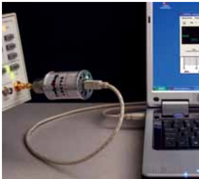
Fig. 2 In addition to DSOs and data-acquisition units, USB instrumentation provides RF and microwave test capabilities such as power meters and synthesized sources. Courtesy of LadyBug Technologies.
