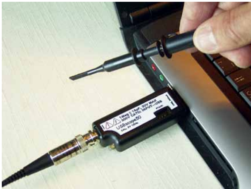
Fig. 1 USB instruments can pack considerable test capability into a tiny package, such as this 50-Msamples/s shirt-pocket digital storage oscilloscope. Courtesy of Elan Digital Systems.
